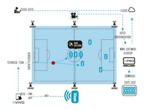
Figure 1 Graphical representation of the UWB data recording and analysis system.
