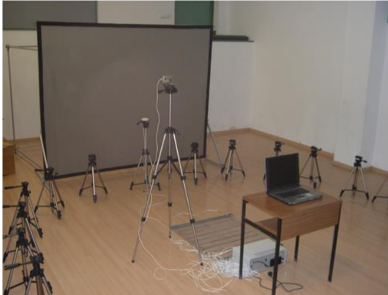
Figure 1. “Pheripherix” system used to assess the reaction response to visual (lights and/or geometrical shapes) and sound stimuli
