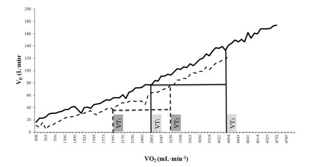
Figure. 1 Procedure for calculating the ITA (sum of the areas of the triangle and rectangle described between  $VT_1$  and  $VT_2$  under the curve), in this case for the function  $VO_2/V_E$ . Cyclist (continuous lines) vs. student (discontinuous lines)
