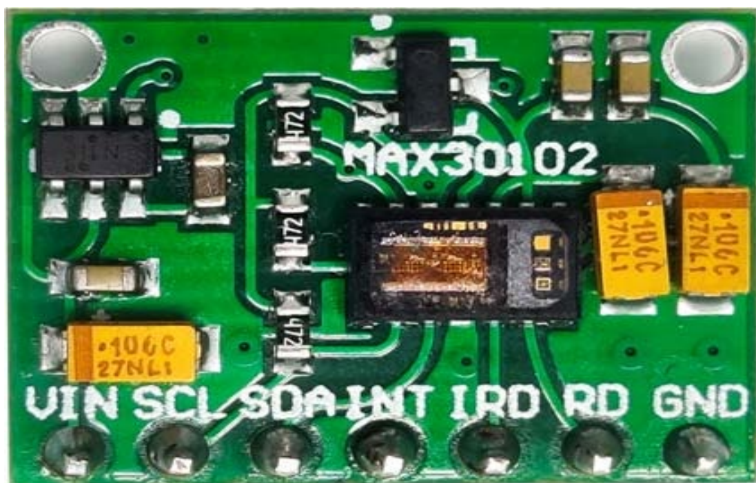
Figure 4. Schematic diagram of the PPG integrated sensor
