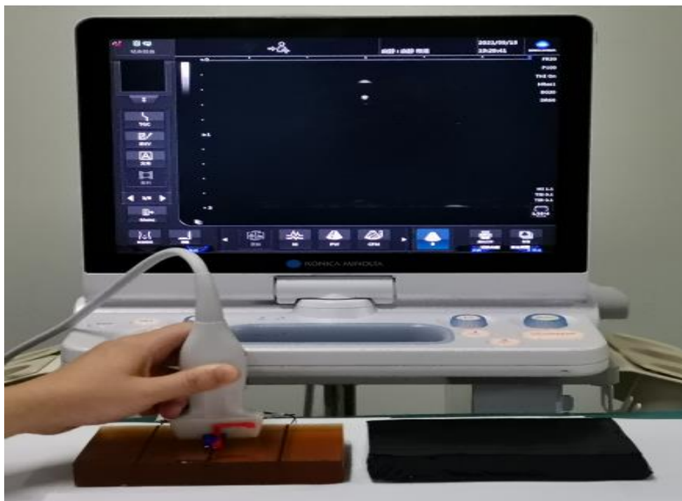
Figure 1: Gelatin phantom with embedded vessels (bright parts on screen are the anterior and posterior walls of the mock vessel). The vessel depth is defined as the distance from the center of short-axis to the surface.
